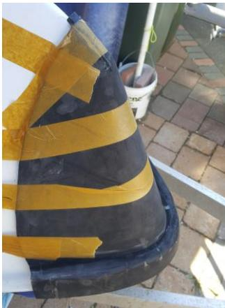
Our prototype solution was a moulded bow protector pad that fits the boat down below the water line protecting the full length of the bow stem. Included is a moulded Vinylester infused fibreglass membrane
